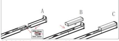
5.Switch right phase and insert modules.
