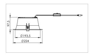
Mateirial: Aluminum casting Leds: OSRAM/PHILIPS Or equvalent Driver: Vossloh Schwabe
