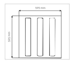
Mateirial: galvanized metal Leds: OSRAM/PHILIPS Or equvalent Driver: Vossloh Schwabe
