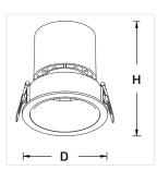
Material: Die-cast aluminum. Embossed aluminum reflector. Driver: VS Led: Philips/ Osram or similar CRI: 90 Optic: 24°, 38°, 55° Body Colour: O Power: 6W/ 12W/ 20W/ 30W Ingress Protection Rating: IP20 CCT: 3000K / 4000K Mounting Type: Recessed ceiling Reflector: White. Additional colors are available upon request: Black, silver, gold, black in matte or glossy shades.
