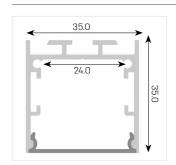
**Material:** Anodized Aluminium. **Diffuser:** Opal / Prismatic.
