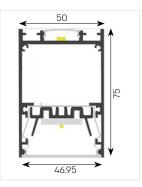
Material: Anodized Aluminium. Coated or Coloured by choice. Diffuser: PMMA / PC Driver: Vossloh-Schwabe. Body Colour: O Additional colours by special order. Optic: Opal. Power: Up to 30W/m CCT: 2700K / 3000K / 4000K Mounting Type: Ceiling mounted / Pendant / Wall mounted. Max Length per Feed: Up to 5 m' for 15W/m model. Up to 3 m' for 30W/m model.
